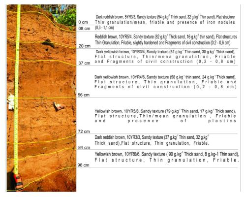
Fig. 5. Profile of Terrigeneous Fluvial Technogenic Deposit, Neblina creek.
