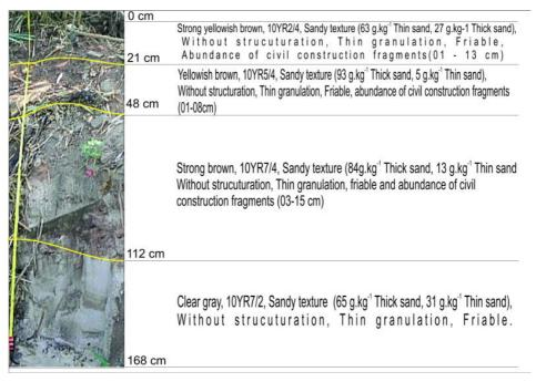
Fig. 8. Profile of inorganic fluvial technogenic deposit, Cimba Creek.
