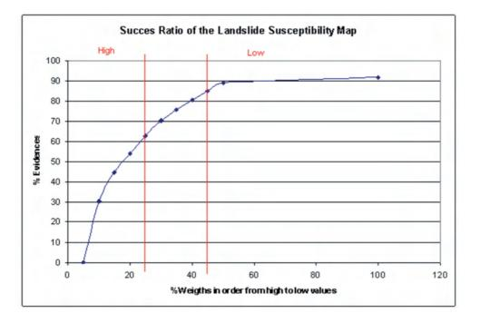
Fig. 5. Success ratio chart showing the predictive capacity of the statistical method when compared with the observed landslides (evidences). The high susceptibility (25% of higher values) areas correlate with 63% of the total mapped landslides.
